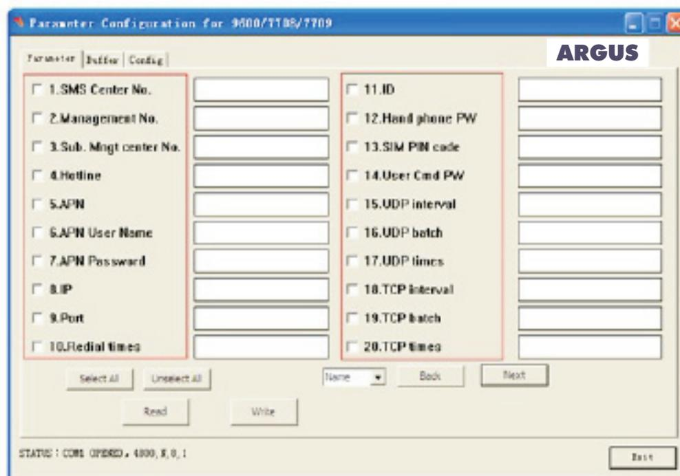
Fill in the APN, IP address, Port, Redial time, SMS center no., Management no. and Sub management no...
