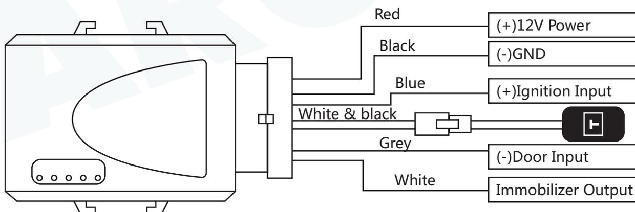
**Red:** Before connecting this wire, remove the supplied fuse. Connect to the battery positive terminal or the constant +12V supply to the ignition switch. Make sure the connection is firmly connected and secure.
