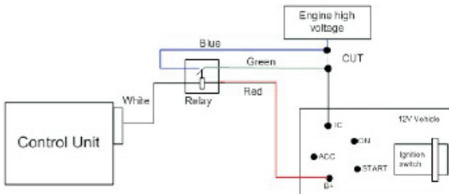
Connect the White Wire with a 32A relay and connects with fuel line or engine power line.
